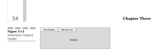
The 8-bit *Next Header* field uses the same values as the field with the same name in the IPv4 header (see Section 3.1.5).
