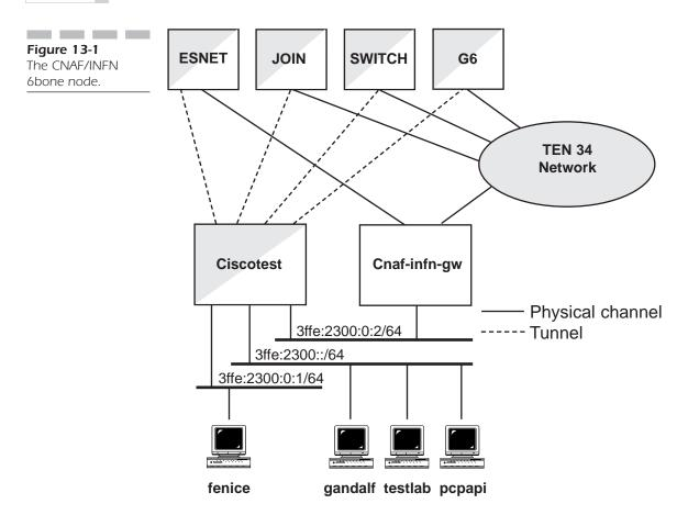
The explanation is based on an example courtesy of the backbone node of 6bone of the Italian research network (GARR), which is run in Bologna by CNAF/INFN<sup>2</sup>. Figure 13-1 depicts the architecture of the 6bone node present at CNAF/INFN (for details, see http://www.cnaf.infn.it).
