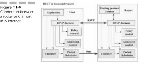
Figure 11-4 Connection between a router and a host in IS Internet
