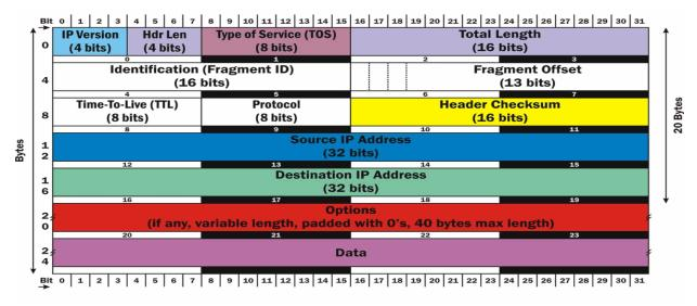
Figure 3.3-b: IPv4 Packet Header
