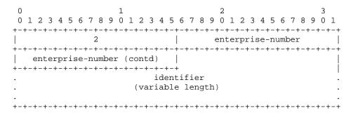
*Link-Layer Address* (DUID-LL) – This type is just like the DUID-LLT, without the timestamp. It is recommended for permanently connected devices that have a link-layer address, but no non-volatile, writeable stable storage.
