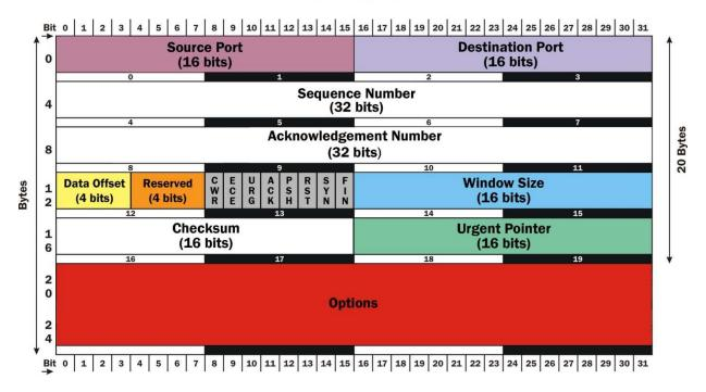
Figure 3.4-a: TCP Packet Header
