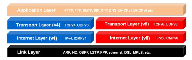
Four Layer Network Model for Dual Stack
