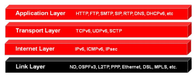
Figure 5.3-a: Four Layer TCP/IPv6 Model
