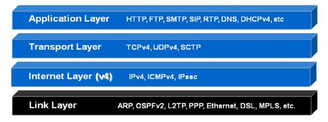
Figure 3.3-a: Four Layer TCP/IPv4 Model
