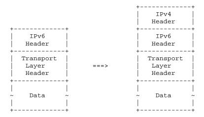
Encapsulating IPv6 in IPv4
