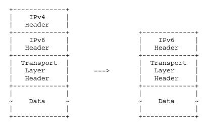
Decapsulating IPv6 from IPv4
