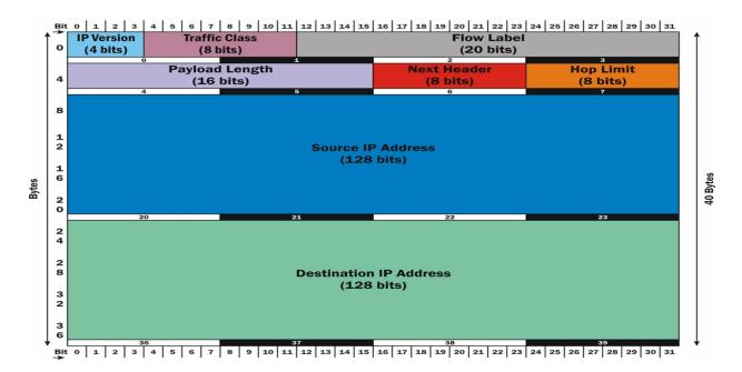
Figure 5.3-b: IPv6 Packet Header
